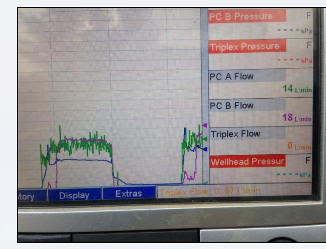
Display of fracture pressures during hydraulic fracturing
